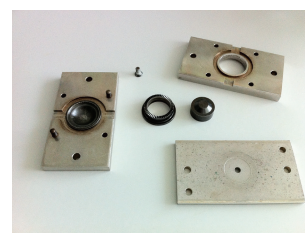
(1) Mold made of stainless steel with diamond-like-carbon (DLC) coating on relevant parts of the topography for capsule production
